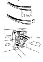
CAUTION: Two speaker systems can be connected to this unit. The minimum speaker impedance should be 4 Ohm when only one speaker system is connected. When two speaker systems are connected, care should be taken that net impedance does not become less than 4 Ohm.
